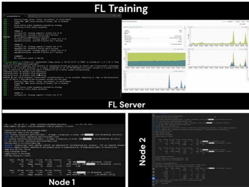
Figure 67: Overview of the FL process. Top panel: the FL Server terminal along with its usage metrics and statistics. Bottom panel: Node 1 and Node 2 perform training on their local data and the server aggregates the results after each round.
