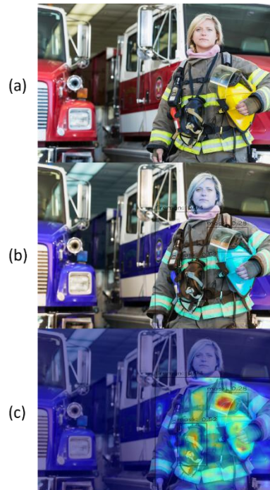
Figure 39: (a) Initial image for Personal Protective Equipment (b) Detected Protective Equipment Objects (c) Eigen-CAM Protective Equipment Objects Analysis
